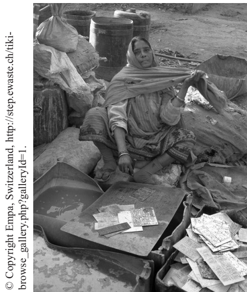
A woman in India recovers metals from circuit boards using an acid bath process.
