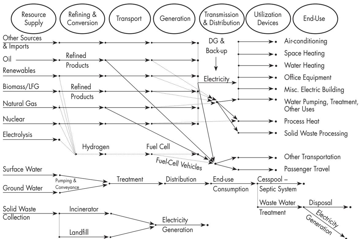
FIGURE 1. MARKAL REFERENCE ENERGY SYSTEM WITH WATER, WASTE WATER, AND SOLID WASTE SYSTEMS
